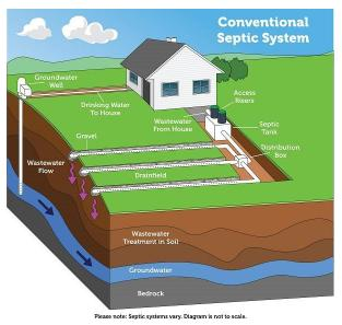
In a conventional OSTDS, a septic tank does not reduce nitrogen from the raw sewage. In Florida, approximately 30-40 percent of the nitrogen levels are reduced in the drainfield of a system that is installed 24 inches or more from groundwater.<sup>42</sup> This still leaves a significant amount of nitrogen to percolate into the groundwater, which makes nitrogen from OSTDSs a potential contaminant in groundwater.<sup>43</sup>
