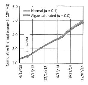
Figure 8: Estimated algae effect on estimated cumulative heat rejection rate from the power plant
