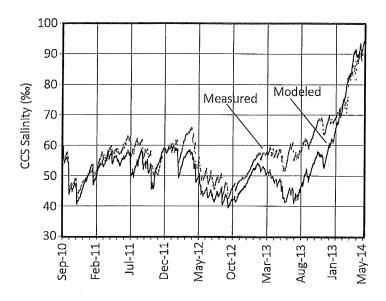
Figure 14: Measured and modeled salinity variations in CCS
