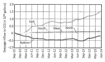
Figure 12: Seepage into CCS from aquifer
