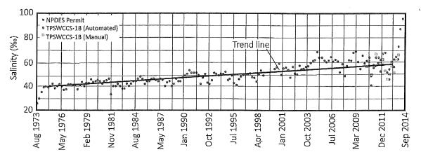
Figure 10: Maximum observed salinities in the CCS since initial operation
