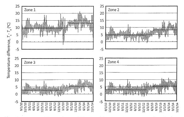
in Figure 9, where the average temperature difference during Period 1 and Period 2 are shown as horizontal lines. It is apparent from Figure 9 that the increase in the average heat-rejection rate from Period 1 to
