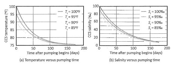
Figure 16: Approximate effect of pumping 100 mgd on temperature and salinity in CCS
