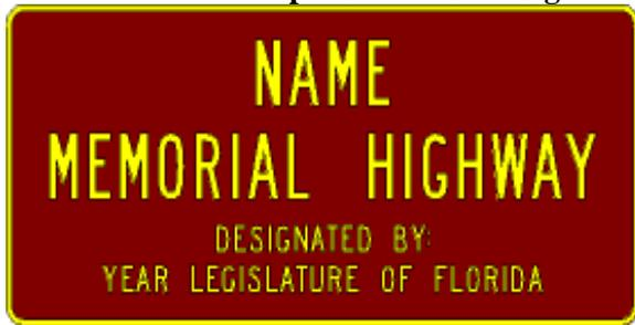
The FDOT sign fabrication facility in Lake City manufactures all approved highway signs for the FDOT, including road designation signs, for use on state roads. According to the department's Traffic Engineering Manual, the signs used for memorial roadway designations shall be a brown panel with yellow lettering as shown in Exhibit 2.
