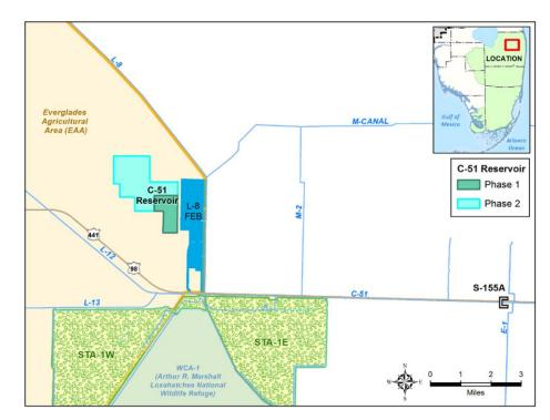
Phase I of the project will provide approximately 14,000 acre-feet of water storage and will be connected hydraulically to the adjacent L-8 Flow Equalization Basin, which is part of the SFWMD's regional system for conveying and managing water.<sup>3</sup> The SFWMD has designated Phase I as a pilot alternative water supply project, and the project is located in the Lower East Coast Regional Planning Area, in a restricted allocation area.<sup>4</sup> Water from Phase I will be
