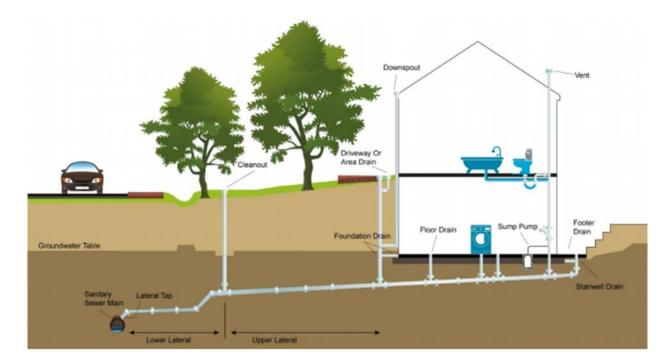
Sanitary sewer laterals are often in poor condition and defects can occur due to aging systems, structural failure, lack of maintenance, or poor construction and design practices.<sup>37</sup> Problems in sanitary sewer laterals can have a significant impact on the performance of the sewer system and
