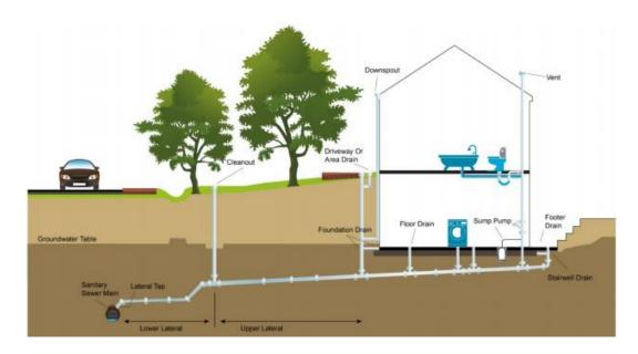
Sanitary sewer laterals are often in poor condition and defects can occur due to aging systems, structural failure, lack of maintenance, or poor construction and design practices.<sup>4</sup> Problems in sanitary sewer laterals can have a significant impact on the performance of the sewer system and treatment plant and can account for half of the infiltration and inflow to sanitary sewers.<sup>5</sup> Cracked or broken laterals can allow groundwater and infiltrating rainwater to enter into the
