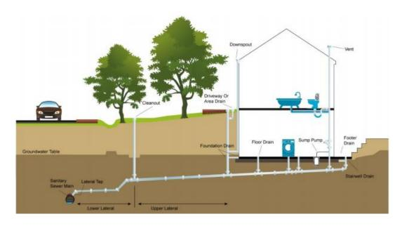
Sanitary sewer laterals are often in poor condition and defects can occur due to aging systems, structural failure, lack of maintenance, or poor construction and design practices.<sup>3</sup> Problems in sanitary sewer laterals can have a significant impact on the performance of the sewer system and treatment plant and can account for half of the infiltration and inflow to sanitary sewers.<sup>4</sup> Cracked or broken laterals can allow groundwater and infiltrating rainwater to enter into the
